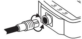
ROTATE CONNECTOR TO MATCH THE GROOVE WITH THE KEY AND PUSH IN.
